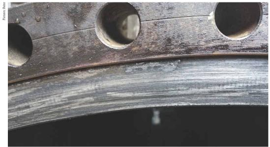
Clean sealing surfaces are a basic prerequisite of an optimally functioning flange system. Contamination of the kind shown here must therefore be completely removed.
